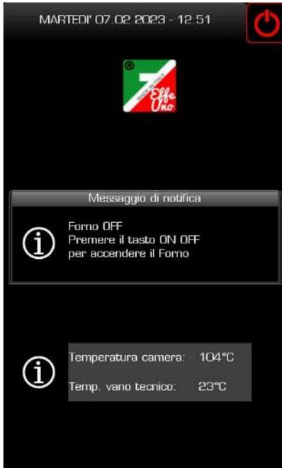
To turn the oven on, tap and hold the ON/OFF
